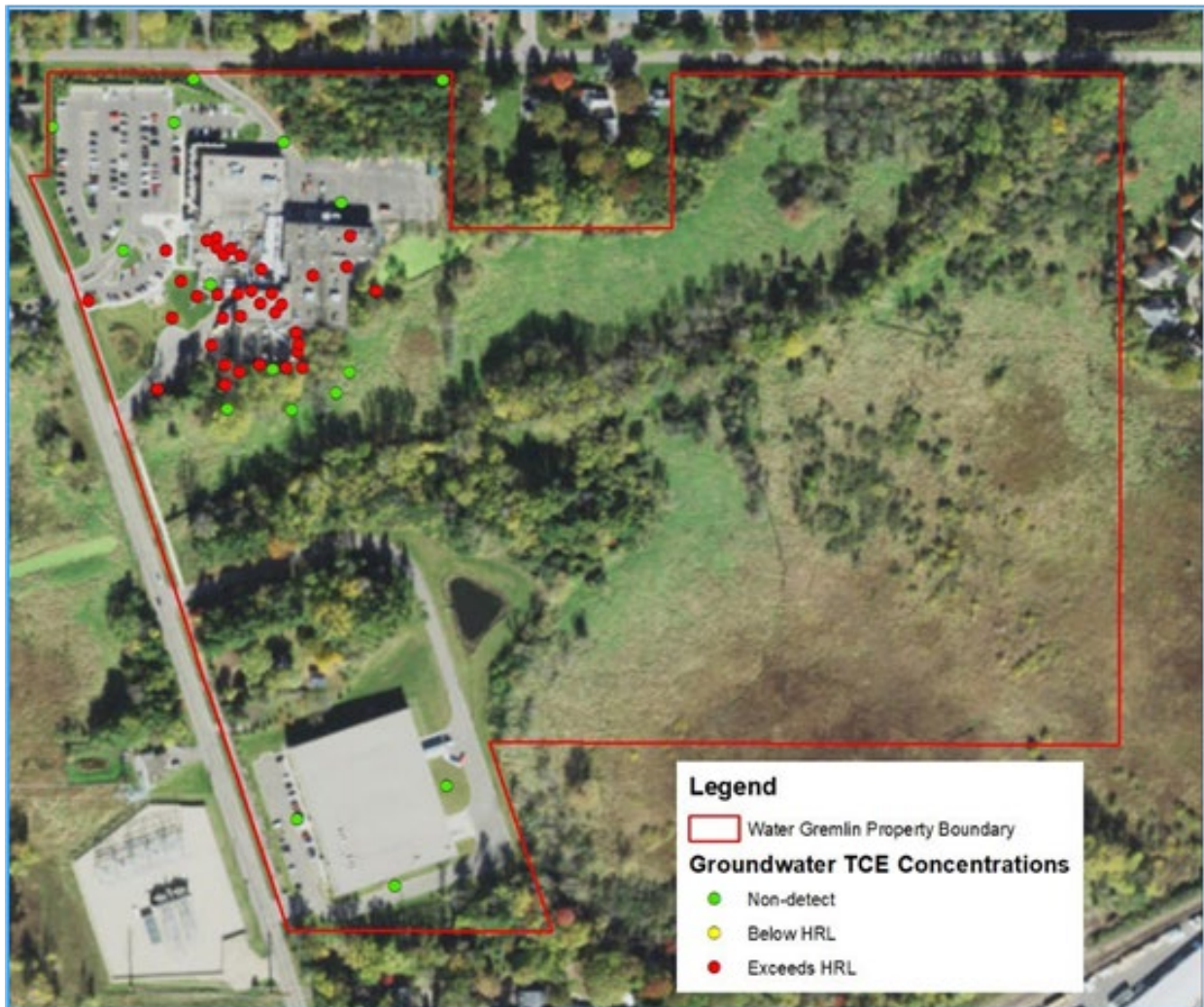
Figure 5: TCE in Groundwater Sampling Results
