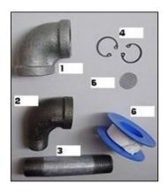
If extra height is not needed, two street elbows (#2) may be used and numbers 1 and 3 above are not needed. Screw an internal ring clamp into the street 90° elbow stopping before the end of the threads. Carefully press the screen into place and secure using second internal ring clamp. Next, remove plug from well cap and assemble the nipple and two elbows on the well seal as shown. Use pipe tape, or compound on the threads.
