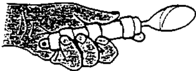
E. CUTLERY WITH BUILT-UP HANDLES FOR EASIER GRIPPING; MOVABLE GRIP RINGS ADJUST FOR COMFORT
